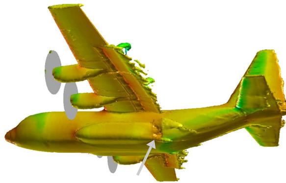
Figure 10: DES prediction of flow over the C-130H with paratroop doors open. Isosurface of vorticity colored by pressure.
