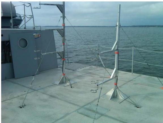
**Figure 4. Ultrasonic anemometers installed on YP676 flight deck.**
