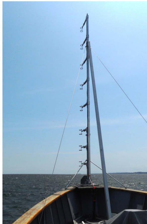
**Figure 5. Bow anemometer array. Reference anemometer is third from bottom.**
