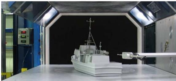
**Figure 6. 4% scale YP model in USNA wind tunnel.**
