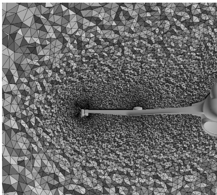
Figure 4: Crinkle cut plane through the grid at FS496 (fuselage station on airplane in inches, positive aft).
