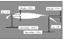
Figure 1. NACA 63<sub>2</sub>-215 Mod. B airfoil section with slat and Fowler flap.
