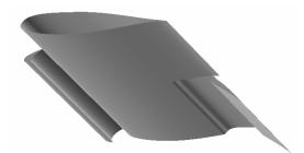
Figure 2. Part-span flap/part-span slat wing geometry.
