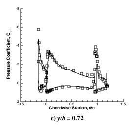
Figure 9. Comparison of computed surface pressures and experimental data at three spanwise locations (? experimental data, ? numerical prediction).
