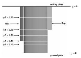
Figure 3. Part-s pan slat/part-span flap wing (y/b locations are noted for pressure tap locations that are considered in this study).
