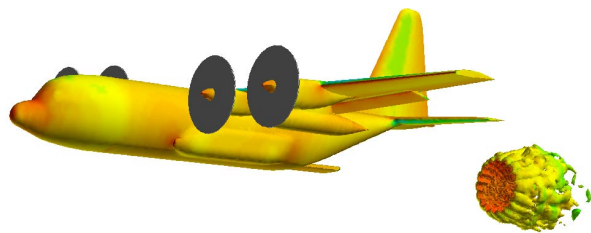
Fig. 13 Iso-surface of vorticity on a 15ft extraction chute behind a C-130H.
