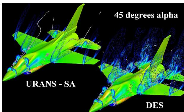
**Fig. 10** DES predictions of the flow over the F-16 at  $45^\circ$  angle-of-attack – DES vs. Unsteady RANS. The surface is colored by pressure, contours are of vorticity, and gray filaments are auto-detected vortex cores.
