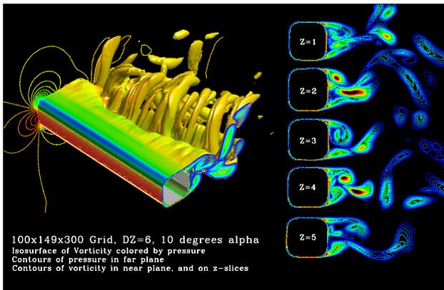
Fig. 2 DES prediction of the flow over a rounded-corner square at  $Re = 800,000$ .
