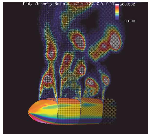
**Fig. 7 DES prediction of flow over a three-dimensional forebody at 90° angle-of-attack.**
