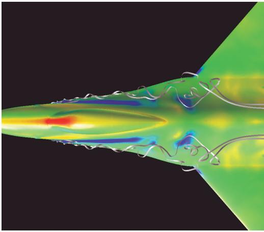
**Fig. 11** DES prediction of flow over the F-16 at 45° angle-of-attack – surface colored by pressure, and streamlines.
