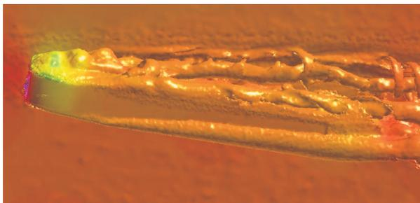
**Fig. 8** DES prediction of the flow over a notional tractor-trailer – isosurface of vorticity colored by pressure
