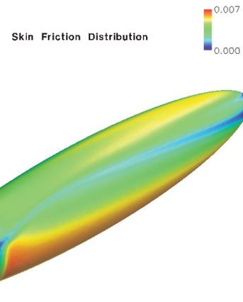
**Fig. 6 DES prediction of the flow over a prolate spheroid. Skin friction contours shown for the flow at 20° angle of attack.**
