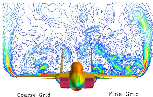
**Fig. 14** Instantaneous vorticity contours at 680 inches behind the aircraft reference point. Coarse-grid prediction in left-half plane, fine-grid result in right-half plane.
