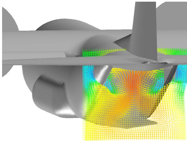
**Fig. 9** Laminar simulation of the C-130 with back door open – vectors colored by upward component of velocity
