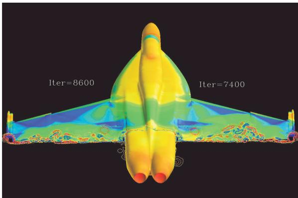
**Fig. 12** DES prediction of flow over the F/A-18E – surface colored by pressure, and contours of vorticity.
