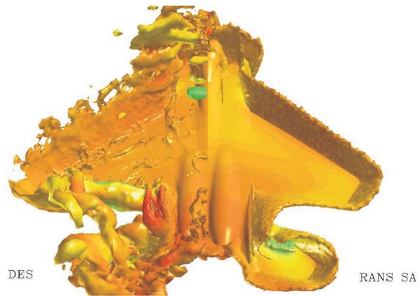
**Fig. 13** DES prediction of flow over the F-15E at 65° angle-of-attack – DES vs. RANS. Isosurface is of vorticity colored by pressure.
