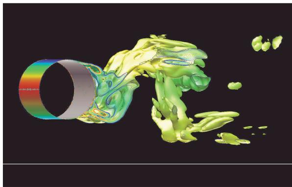
**Fig. 1** DES prediction of the flow over a circular cylinder at  $Re = 800,000$ . Isosurface of vorticity colored by pressure.
