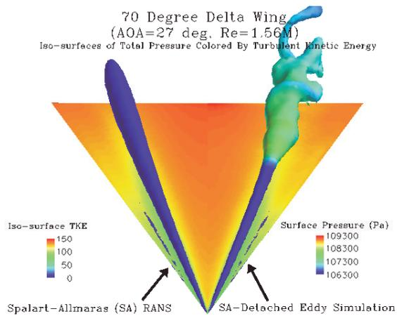
Fig. 3 DES prediction of the flow over  $70^\circ$  swept delta wing.
