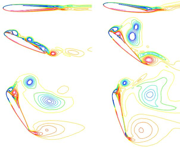
**Fig. 5 Unsteady pitch up of a NACA 0012 airfoil – contours of vorticity.**
