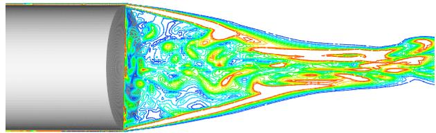
Fig. 4 DES prediction of flow over an axisymmetric base at Mach 2.46. Contours of vorticity.
