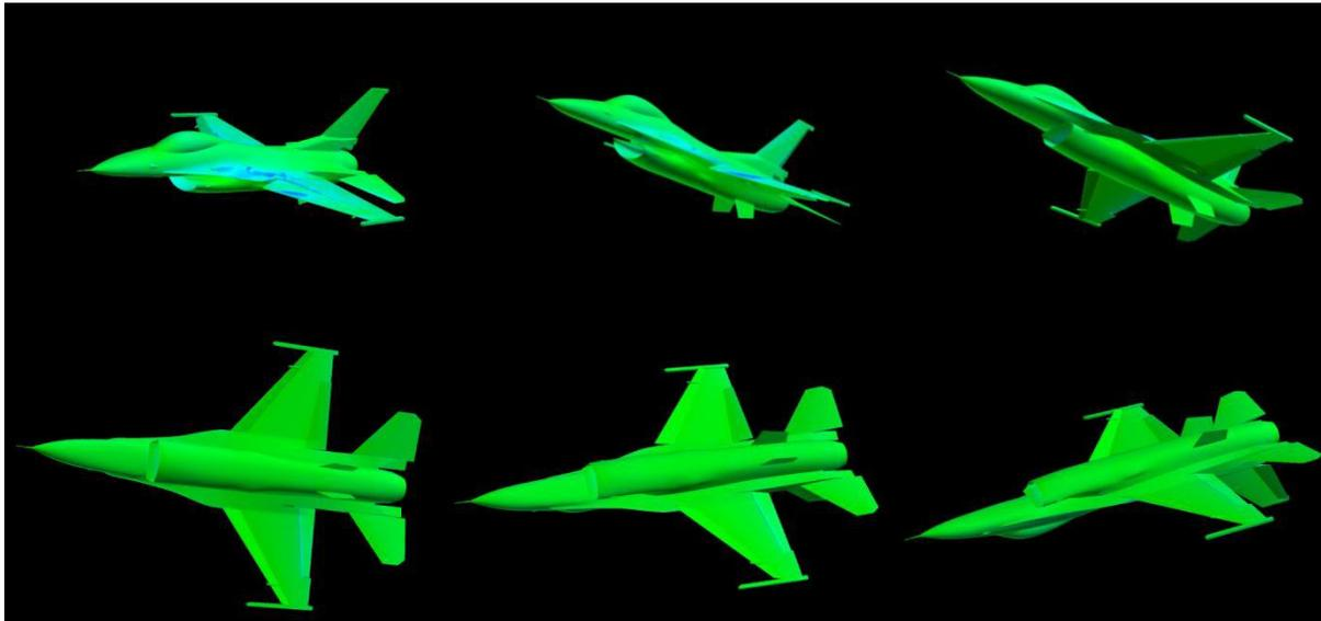
**Figure 6. F-16 Loaded Roll CFD simulation at Mach 0.6 and 10,000 feet.**
