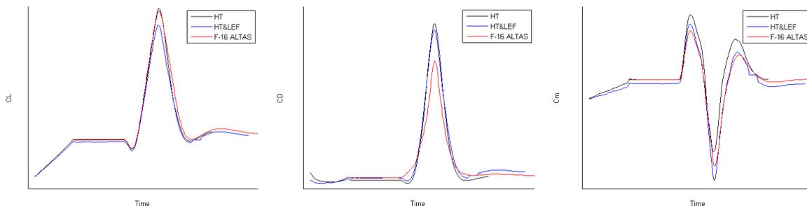
**Figure 5. F-16 Pitch Doublet CFD simulation with moving HTs and LEFs at Mach 0.6 and 10,000 feet.**
