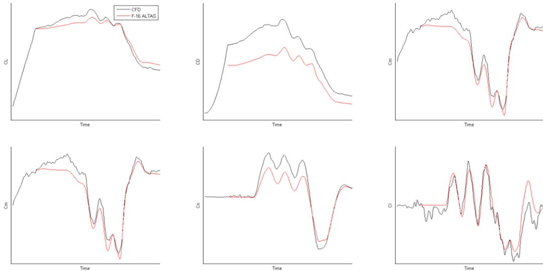
Figure 7. F-16 Loaded Roll CFD simulation with moving control surfaces at Mach 0.6 and 10,000 feet.
