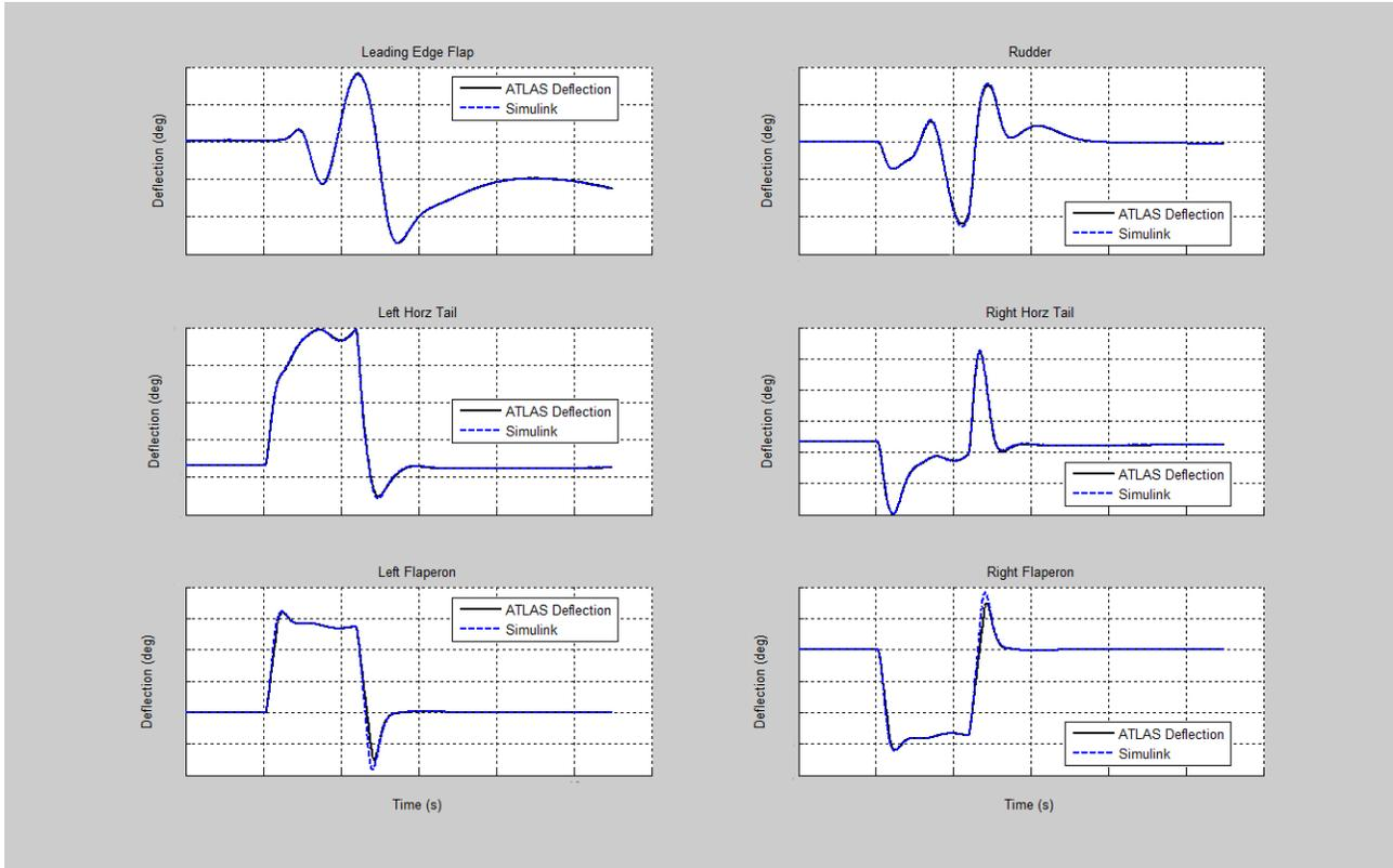
**Figure 9. Right Roll 360 degree at 0.6 Mach and 10,000 Feet**
