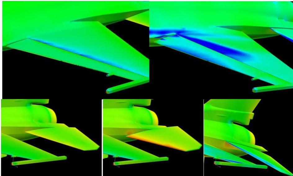
**Figure 4. Overset Grid of Clean F-16 during a pitch doublet with moving horizontal tails and LEFs at Mach 0.6 and 10,000 feet.**
