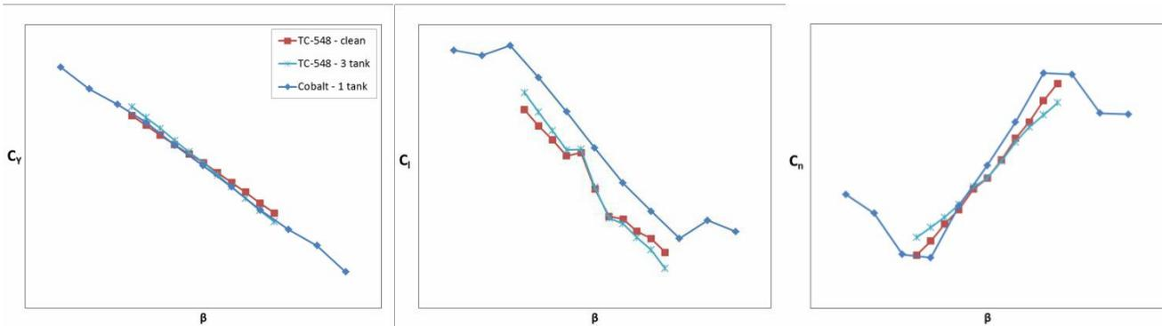
Figure 3. A-10 Static CFD data vs. wind tunnel data at Mach 0.65
