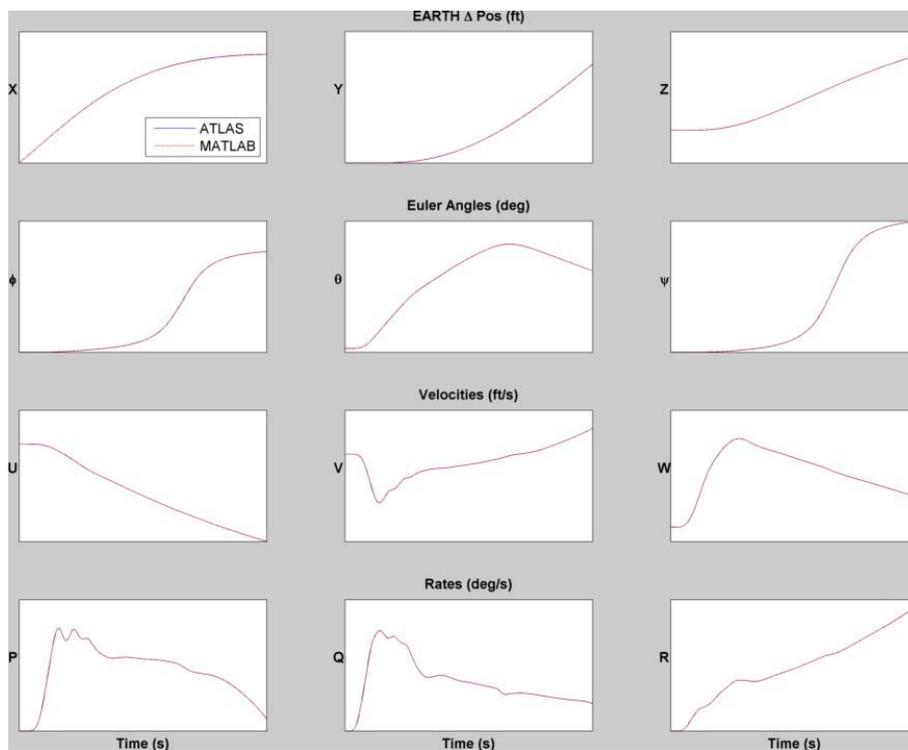
Figure 8. 6-DoF comparison, MATLAB vs. ATLAS, Max G Pull-up, Mach 0.6 at 10,000 ft.
