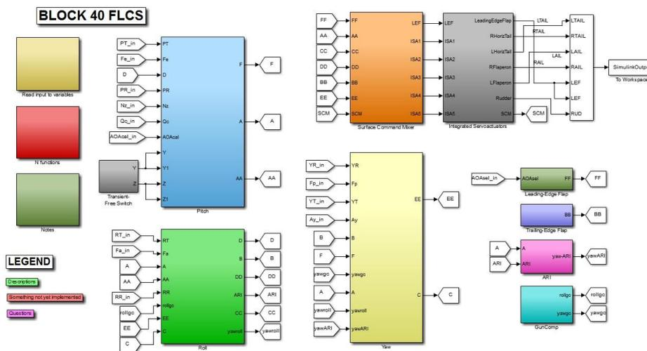
Figure 1. F-16 FLCS logic modeled in Simulink.
