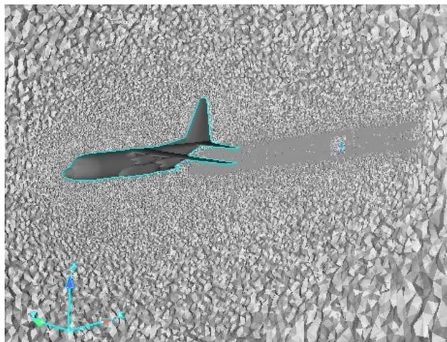
**Figure 5. Combined Geometry and Computational Grid of aircraft (C-130) and Drogue Parachute Grids.**
