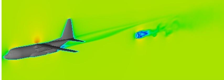
**Figure 8. Detail of combined aircraft Speed in flowfield (C-130) and drogue parachute domains.**
