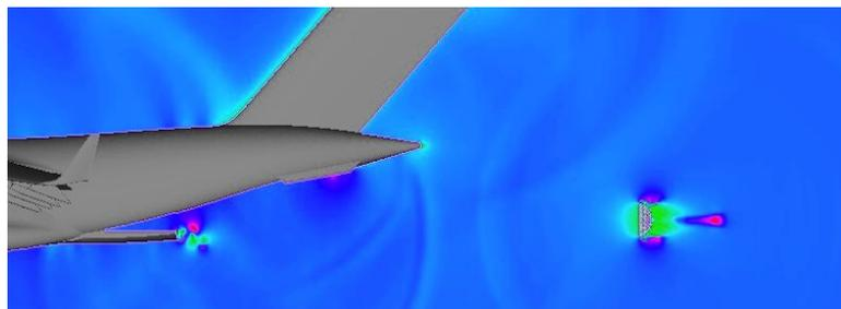
**Figure 10. Dynamic pressure field detail immediately aft of the aircraft (C-17).**
