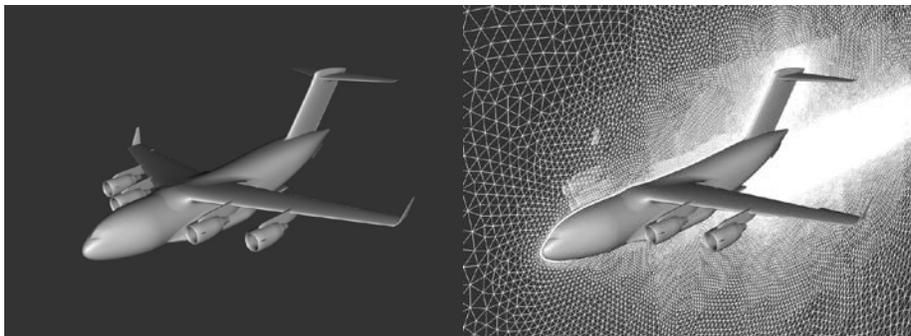
**Figure 2. Computational Geometry and Computational Grid around the C-17 aircraft.**
