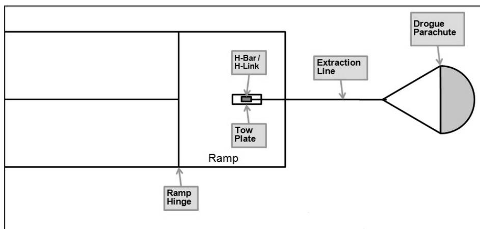
**Figure 7. Tow Plate schematic of Drogue Parachute in tow configuration.**
