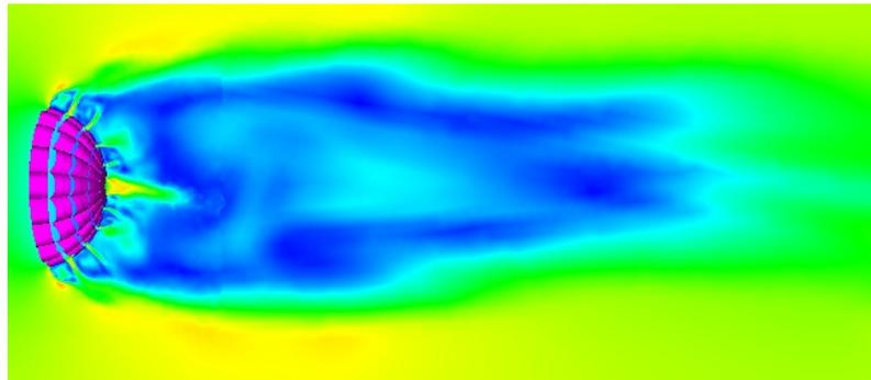
**Figure 9. Detail of Speed in flowfield local to the Drogue Parachute.**
