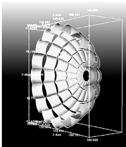
**Figure 3. Computational Geometry and Computational Grid Domain for the ring-slot Drogue Parachute used.**
