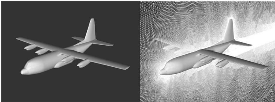
**Figure 1. Computational Geometry and Computational Grid around the C-130 aircraft**
