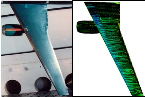
**Figure 30: Experimental and computational oil flow image of upper wing.**
